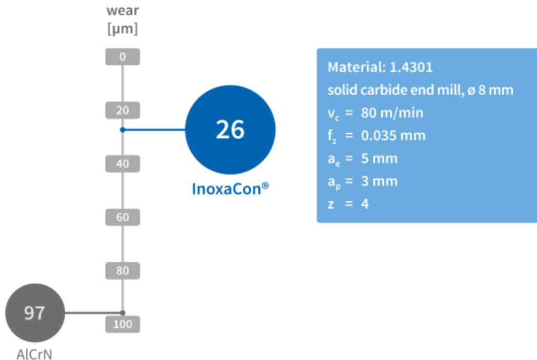
A practical example in comparison with AlCrN underscores the efficiency of the HiPIMS coating material.
