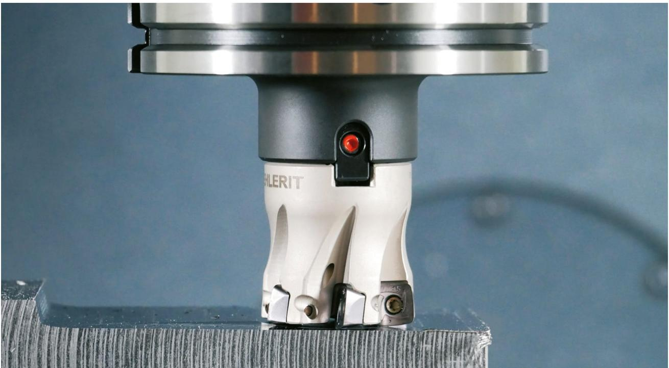
The new FerroCon® coating specifications enable faster milling with significantly increased tool service life and improve the quality of the workpiece surfaces produced. (Photo: Boehlerit GmbH & Co. KG)
