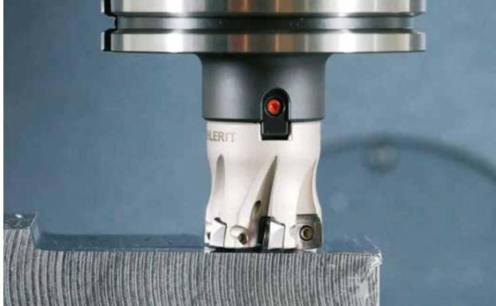
The new FerroCon® coating specifications enable faster milling with significantly increased tool service life and improve the quality of the workpiece surfaces produced. (Photo: Boehlerit GmbH & Co. KG)
