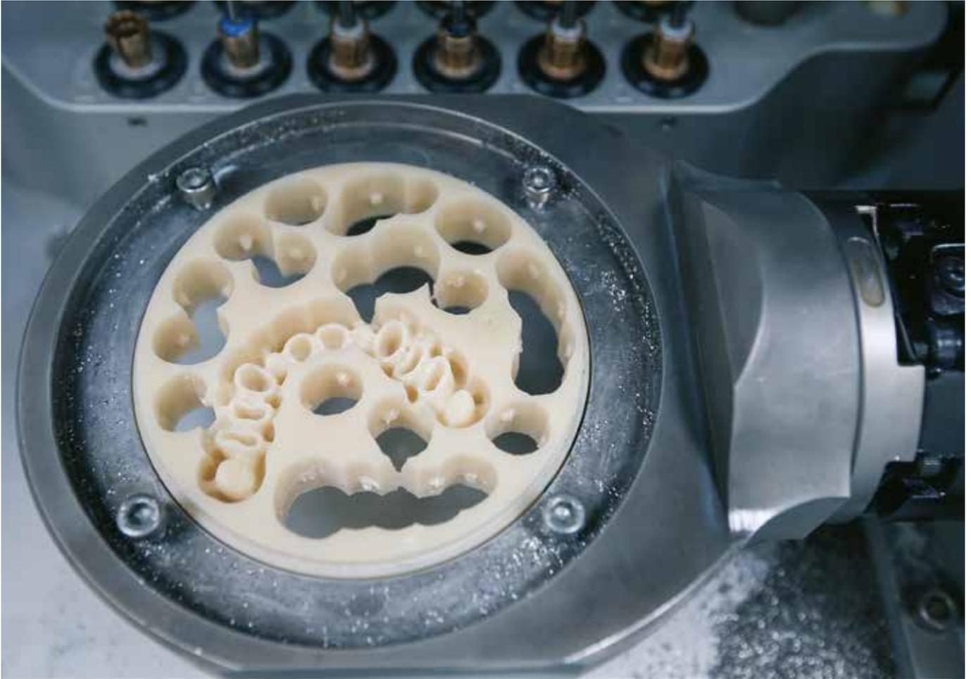
Known as the green compact (before the ceramics are fired), zirconium oxide is highly abrasive and porous at the same time. The wear resistance of cutting tools presents challenges to processing.
