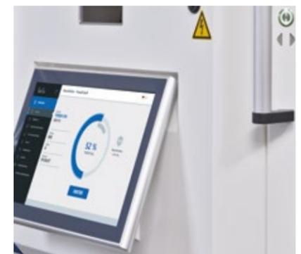
Intuitive touch control and pneumatic actuators for chamber doors facilitate daily operation of the unit.
