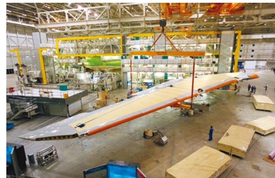
Composite airplane wings, drilling and reaming the rivet holes with diamond-coated tools
