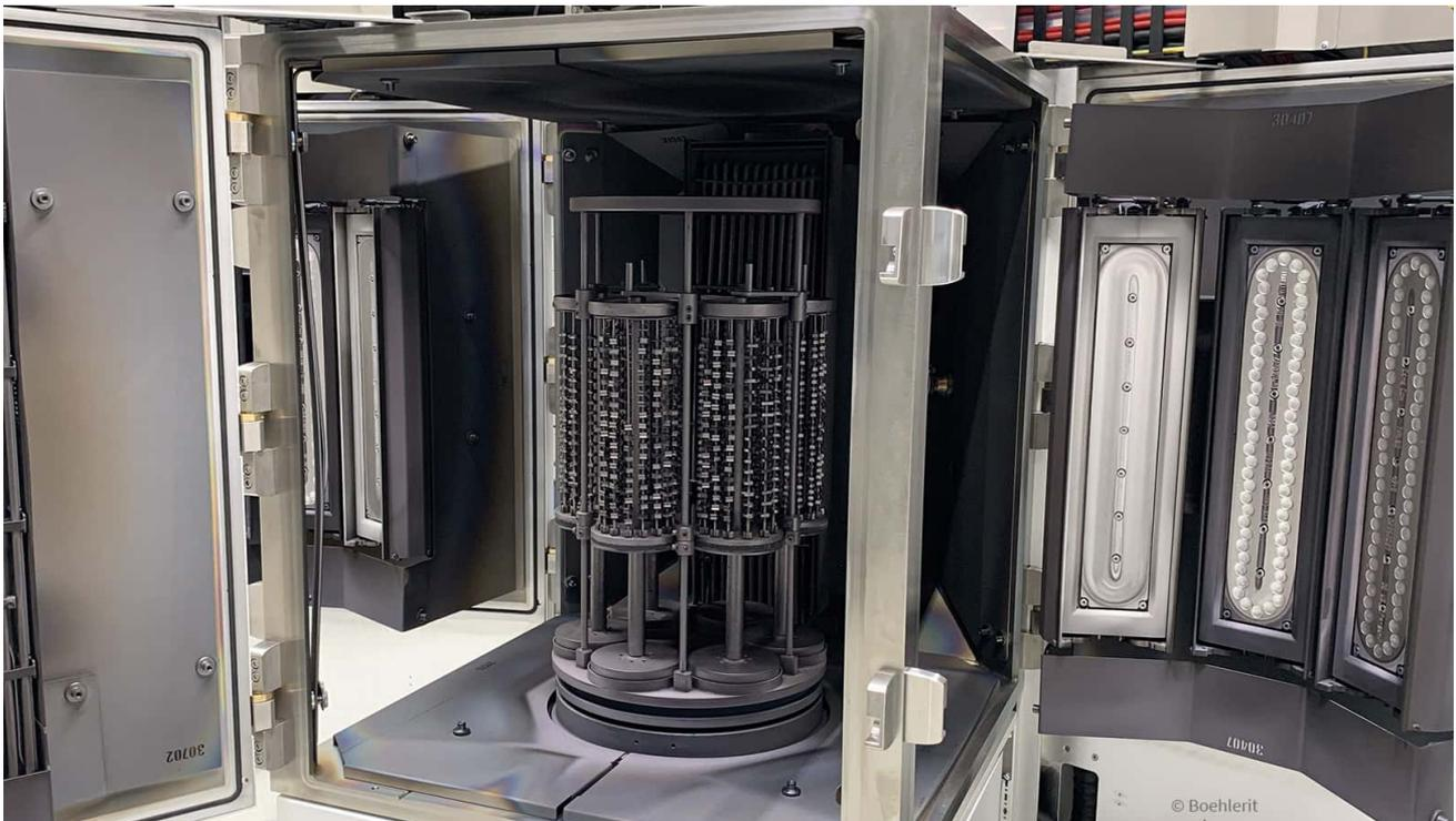
HiPIMS enables coating thicknesses of up to 12  $\mu\text{m}$  and also significantly increases the quality and performance of the coatings.
