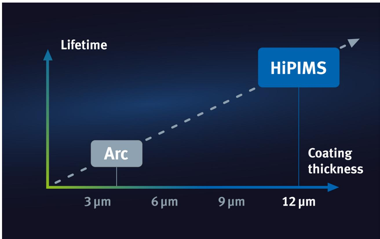
12 µm coating thickness – a new horizon in coating technology for cutting inserts.
